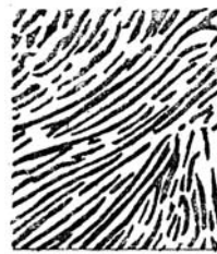
Fig. 8.2 Micro structure of pearlitic eutectoid steel
